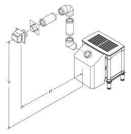
Figure 27 - Horizontal Termination Configuration for Rigid Venting Using One  $90^\circ$  Elbow
